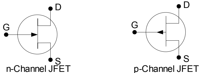
Drawing 17: Schematic Symbols for J-FETs
