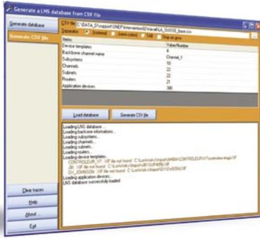
NLCSV is a collection of LNS® Plug-Ins for easy integration and automation of network management functions. It is the perfect complement to NL220 that already implements advanced functions such as automatic download of Configuration Properties and application programs. NLCSV applies rules from an external CSV file to automate integration.
