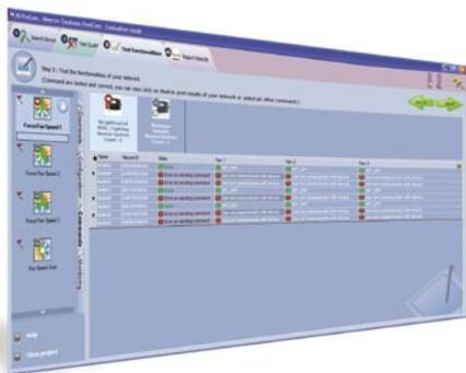
NLPreCom is a highly recommended tool for evaluating the network before the commissioning phase. It is used to verify the wiring of the network, the network topology consistency and the connection of the nodes. This tool is dedicated to technicians on job site who need to prepare the commissioning phase. Reporting functions help the technician to keep the overview at any time in the pre-commissioning phase.
