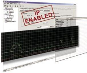
The LOYTEC System Diagnostics Tool (LSD Tool) provides a comfortable user interface to access the network statistics information, which is collected by L-Switch<sup>XP</sup> and L-IP devices. It also allows to remotely configure L-Switch<sup>XP</sup>, L-IP and L-Proxy devices, run parallel firmware upgrades via the network, and provides advanced features like disabling of ports or configuring the management port on L-Switch<sup>XP</sup> devices.
