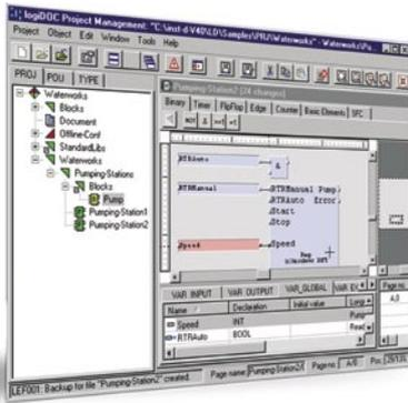
The LINX-110/-111 Automation Server is a CEA-709 compliant programmable device incorporating a set of automation functions and IEC61131-3 function block programming using the logi.CAD programming tool suite.
