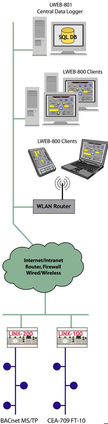
L-WEB uses standard WEB technologies to visualize and control data provided by one or multiple LINX-100 or LINX-200 Automation Servers on a Windows PC or mobile devices like PDA's or Smart Phones running Windows Mobile .
