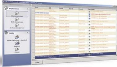
NLTestChannel TE is a background application that continuously checks the quality of the network and proposes actions on how to repair detected errors.
