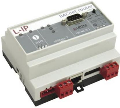
The LIP-ME201 BACnet/IP Router connects a BACnet MS/TP channel to a BACnet/IP network. It routes BACnet packets back and forth through an IP based network, such as a LAN (Ethernet), an Intranet, or even the Internet. The LIP-ME201 is compliant with the standards ASHRAE 135-2004 and ISO 16484-5. LIP-ME201 can be configured to act as a BACnet Broadcast Management Device (BBMD).
