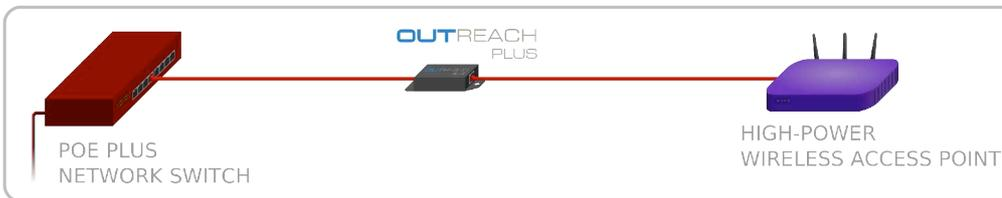
PoE Plus devices such as the 802.11n wireless access point shown in the first example may now be located up to 200 metres from a power source, with no need for expensive mains cable installation for the remote equipment.
