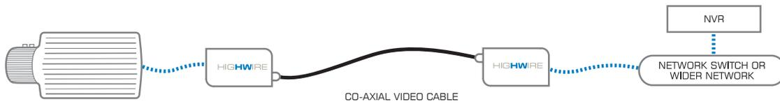
In this application, a high-resolution mega-pixel IP camera replaces a standard analog CCTV video camera. The IP camera's standard Ethernet TCP/IP connection is linked to a HIGHWIRE device with a short CAT5 patch cable (straight-through or cross-over). Both the camera and the HIGHWIRE are powered from the same power supply, and both may be fitted inside a standard external camera housing. The HIGHWIRE link runs across the existing
