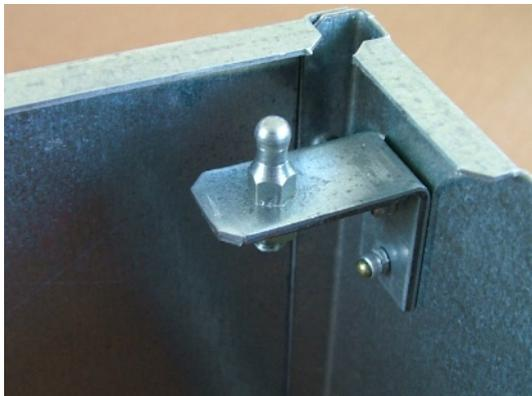
The assembly of the diffuser plate and the base unit is achieved by simple clipping of the two locating lugs into spring clips; demounting is by turning the lugs a quarter turn using a screwdriver.
